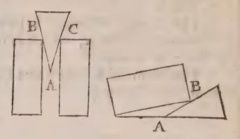
Therefore Vbaldus hath more exactly applyed the severall parts of it according to this form, that the point A, should be as the common fulciment, in which both the sides doe meet, and (as it were) uphold one another; the points B, and C, representing that part of the Leavers where the weight is placed.
